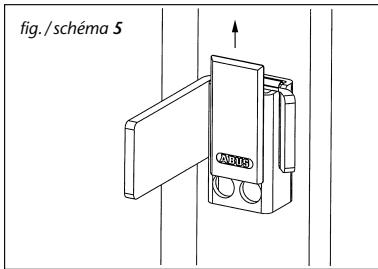
6. Install bolt and allow to engage.
