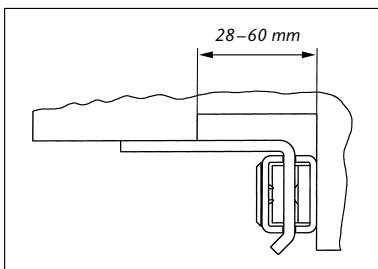
⑥ The ABUS SW 20 Safety Lock effectively protects windows and doors against prying or pushing open from the outside. In case of narrow frames it can be mounted directly on the wall in the recess. Suitable for all windows and doors opening toward the inside with a frame width of 28 up to approx. 60 mm on the handle side. We recommend using two SW 20 Safety Locks on high doors/windows.
