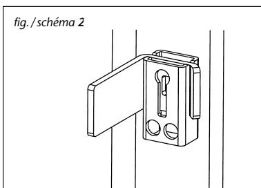
3. Insert dowel and screw on bolt tube through one of the lower holes, see fig. 2.
