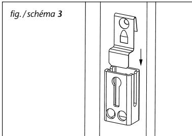
4. Insert catch spring and screw on together with bolt tube (fig. 3).
